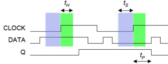
**Setup Time:** DATA must reach its new value at least  $t_s$  before the  $\text{CLOCK}^\uparrow$  edge.
